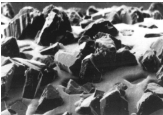
Fig. 6: Grinding layer of an electroplated single-layer diamond wheel in new condition.
