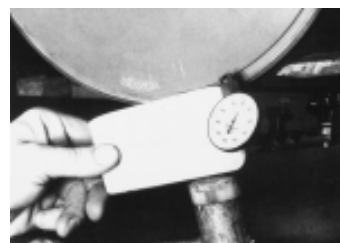
Fig. 10: Adjusting radial runout of a peripheral wheel.
