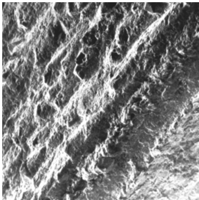
Fig. 7: Grinding layer of a resin-bond CBN wheel in its self-sharpening zone (free-cutting layer).
